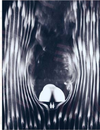
Smoke trails around a hemisphere model (included)
