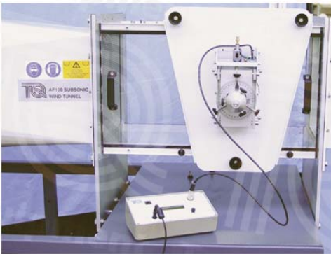
Mounted on side of wind tunnel to measure both lift and drag. Shown fitted with the protractor from the Wind Tunnel.
