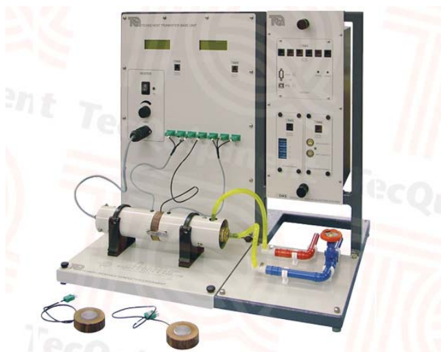
Base unit shown fitted with the optional VDAS-F and the optional Linear Heat Conduction Experiment (TD1002a)
